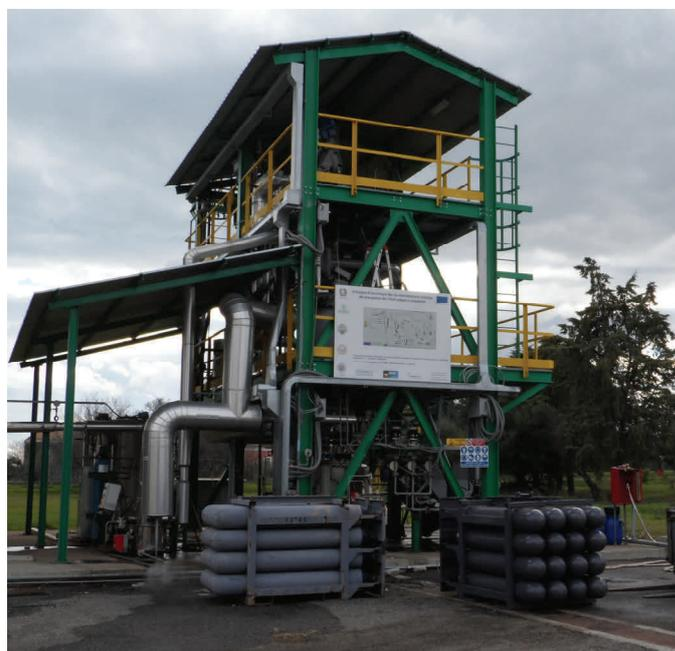
Figure 1: Updraft gasification reactor (PRAGA) at ENEA, Italy.
