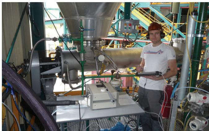
Figure 1: Analyzing tars with IFK's online device at CIUDEN's gasifier.
