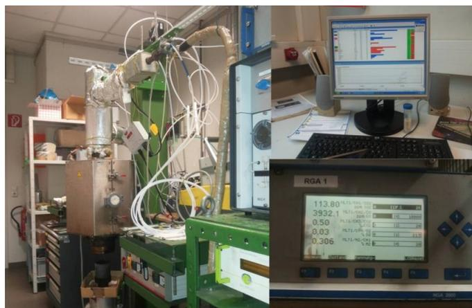
Figure 1: Batch pyrolysis reactor.
