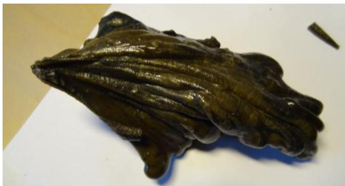
Figure 4: Molten ash (slag) collected from the water quench.
