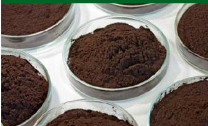
Figure 6: Biocoal from hydrothermal carbonization (HTC) used during the gasification experiments.
