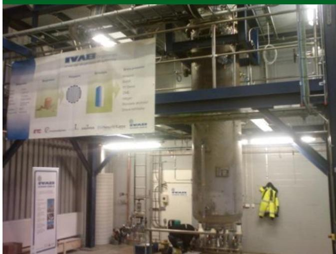
Figure 5: Pressurized Entrained-flow Biomass Gasifier (PEBG) at ETC.
