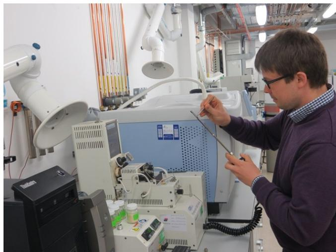
Figure 1: Preparation of a sample for Py-GC-MS analysis.
