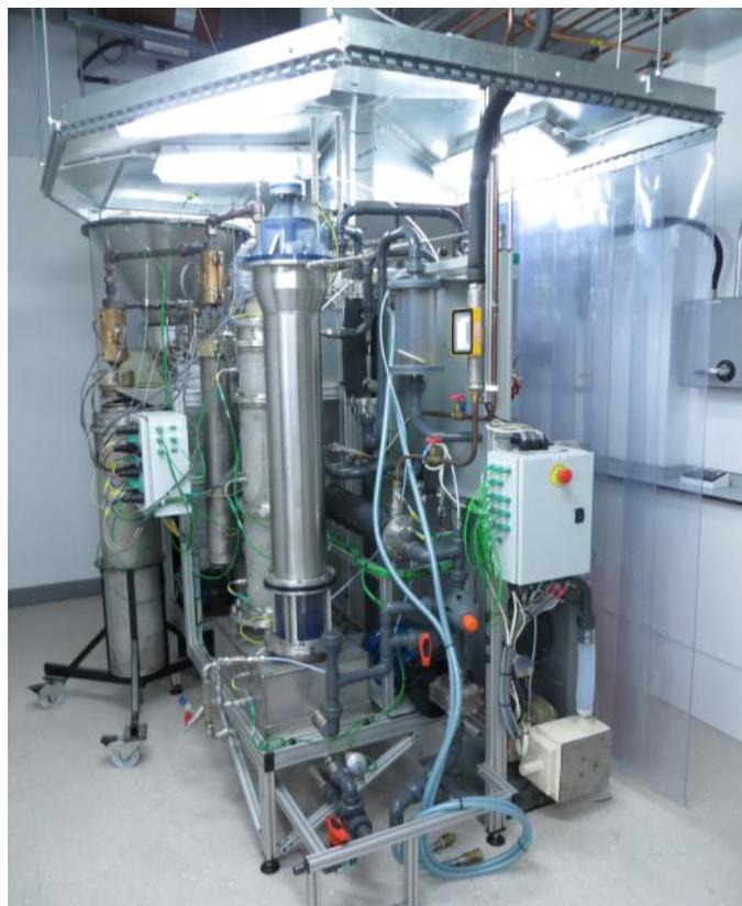
Figure 1: 7 kg/h continuous fast pyrolysis unit.
