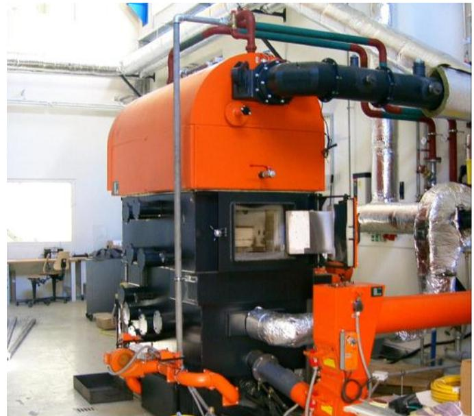
Figure 1: 180 kW<sub>th</sub> grate-fired testing plant.
