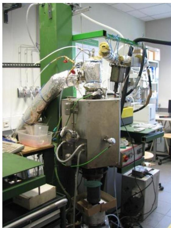
Figure 3: Lab-scale combustion reactor.
