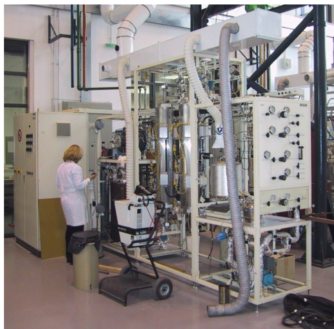
Figure 3: HDS pilot plant unit at CPERI
