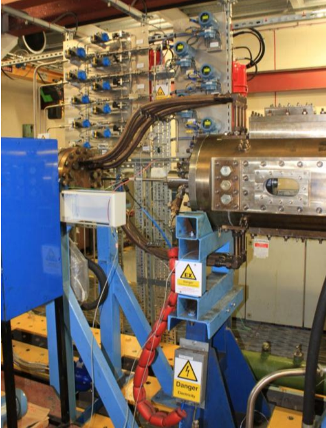
Figure 4: High Pressure Optical Rig shown on the right hand side of the image with the newly designed High Pressure Generic Swirl Burner installed. The syngas fuel board can be seen in the background.
