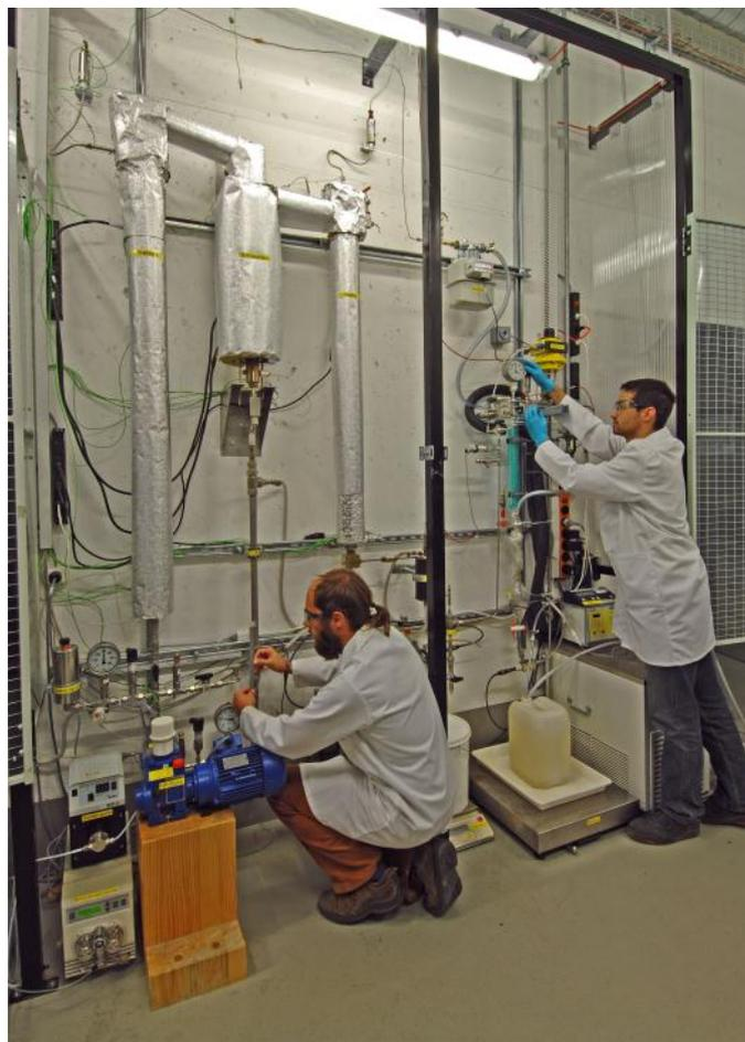
Figure 4: Lab-scale hydrothermal gasifier of wet biomass.
