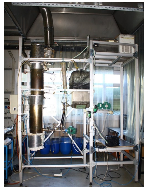
Figure 4: Bench scale bubbling fluidized bed gasifier.
