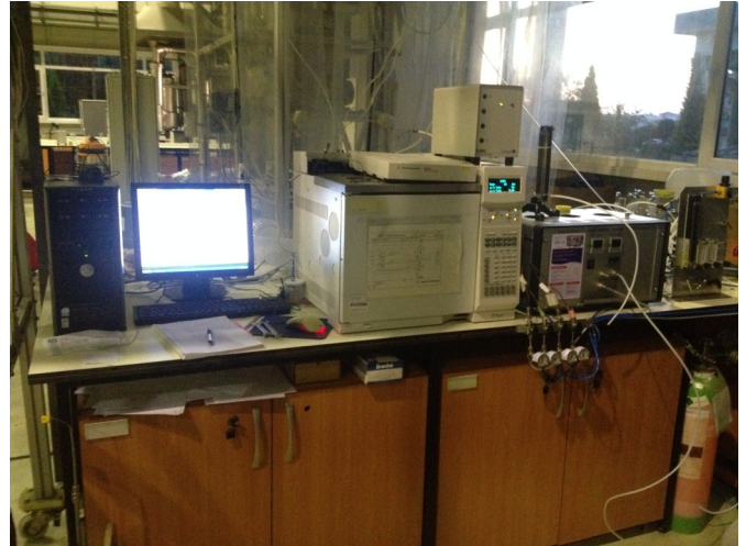
Figure 3: Gas analysis system equipped with gas chromatograph (GC) with pulse flame photometric detector (PFPD) and calibration gas generator.
