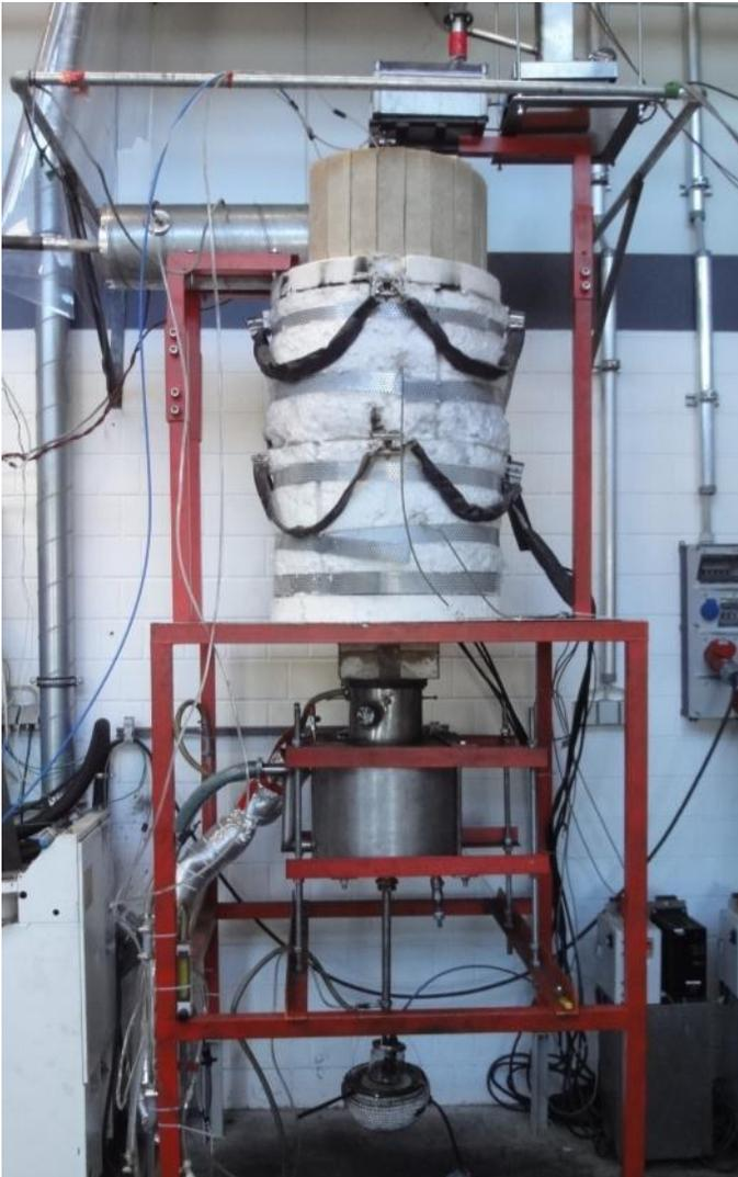
Figure 2: High Temperature Entrained Flow Reactor.
