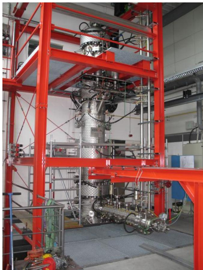
Figure 1: Pressurized High Temperature Entrained Flow Reactor.
