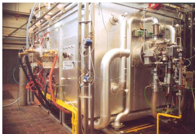
Figure 2: 200 kW High Temperature Air Combustion (HiTAC) test facility.
