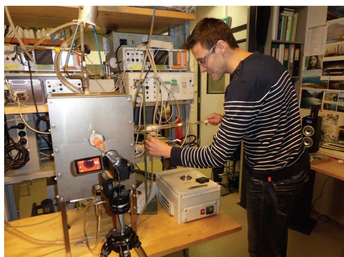
Figure 4: Handling of the Single Particle Reactor (SPR).
