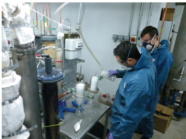
Figure 2: Working on the pyrolysis reactor.
