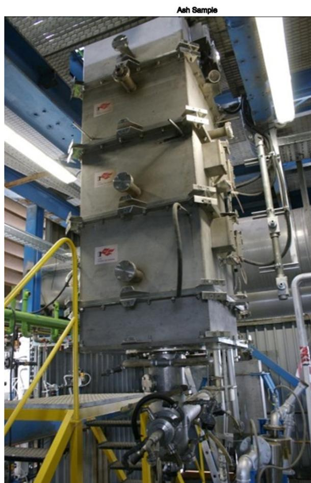
Figure 1: IFRF isothermal plug flow reactor.
