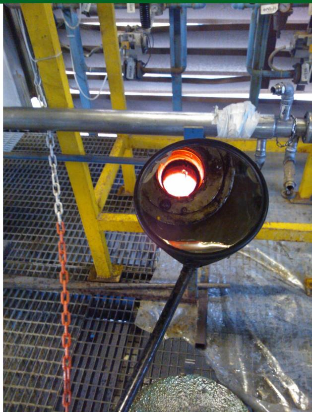
Figure 3: The isothermal plug flow reactor from below - as seen through a mirror.
