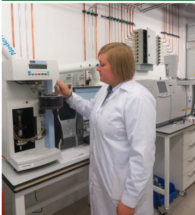
Figure 2: Loading the Thermo-Gravimetric Analyser (TGA).
