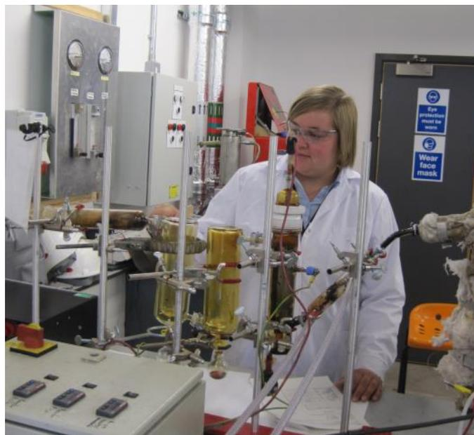
Figure 1: Working with the 300 g h<sup>-1</sup> fluidised bed fast pyrolysis reactor.
