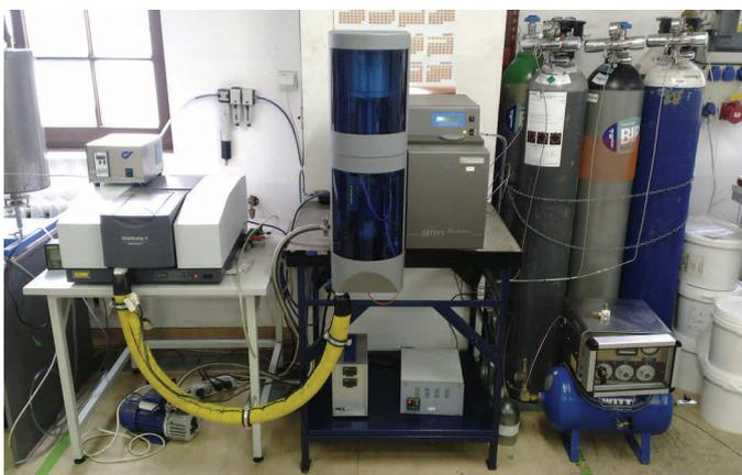
Figure 1: TGA/DSC coupled with FTIR.
