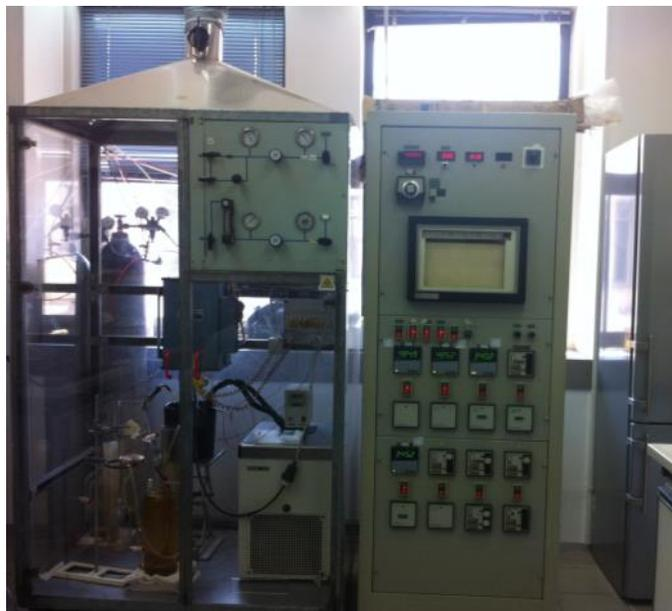
Figure 1: Catalytic pyrolysis unit at CPERI.
