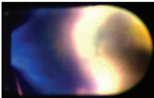
Figure 2: Combustion tests using the saturated biodiesel in the High Pressure Optical Combustor.
