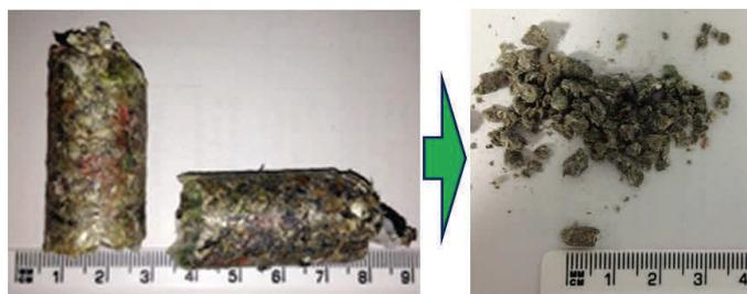
Figure 2: Preparation of RDF pellets to be fed into the WOB reactor: original 4x1.5cm (left); processed 4x3mm (right).
