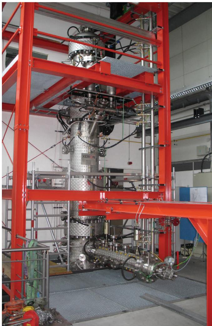
Figure 1: Pressurized High Temperature Entrained Flow Reactor (PiTER).
