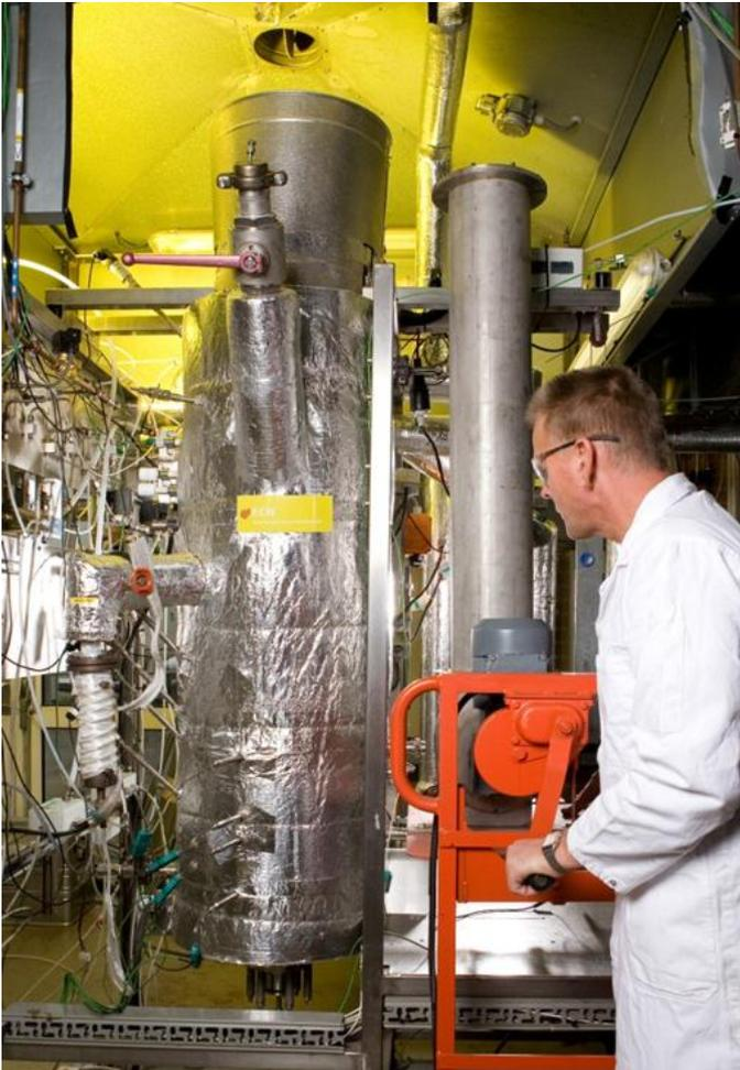
Figure 1: ECN's WOB; suitable for combustion, gasification and pyrolysis experiments.
