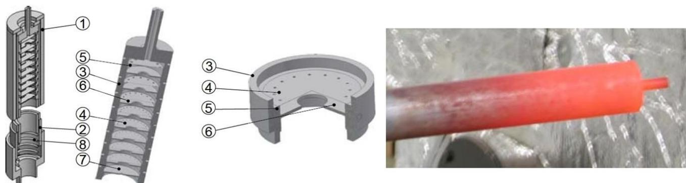
Figure 4: Scheme of the high-temperature impactor (HTI) (left), the HTI directly after taking a measurement (right). Key—1: Outer casing; 2: Inner casing; 3: Shell; 4: Orifice plate; 5: Spacer ring; 6: Stagnation plate; 7: Critical Orifice; 8: Spring.
