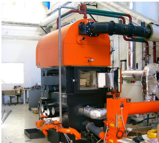
Figure 1: 180 kW<sub>th</sub> grate-fired testing plant.
