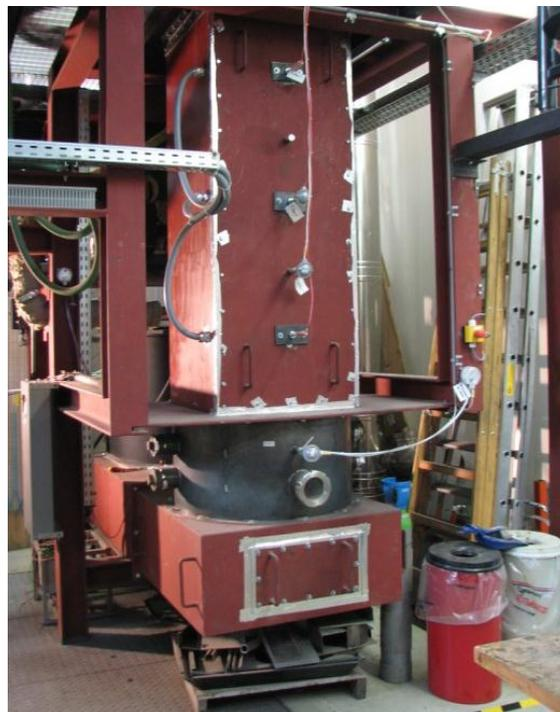
Figure 2: 50 kW grate furnace coupled with a drop-tube furnace.
