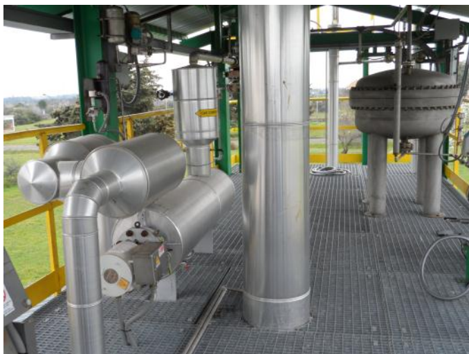
Figure 5: The section for hydrogen enrichment: water gas shift reactor (WGS) - pictured to the left. CO 2 adsorption system based on MEA - pictured right.
