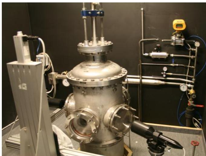
Figure 3: Upper part of the Pressurised Spray Test Rig (PSTR) at ETC and the optical parts of the PDA setup.
