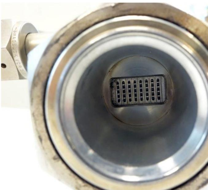
Figure 3: Close-up of a micro-structured reactor used for fuel synthesis (see, for example, R. Myrstad et al., Catal. Today 147S (2009) S301–S304).
