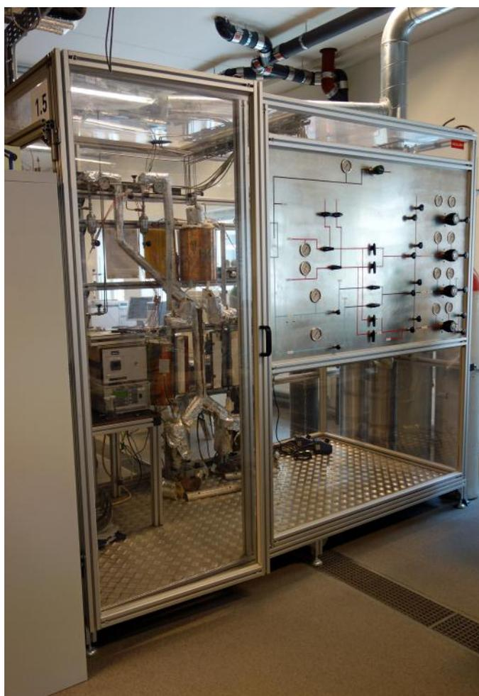
Figure 2: The Fischer-Tropsch synthesis setup for catalyst testing.
