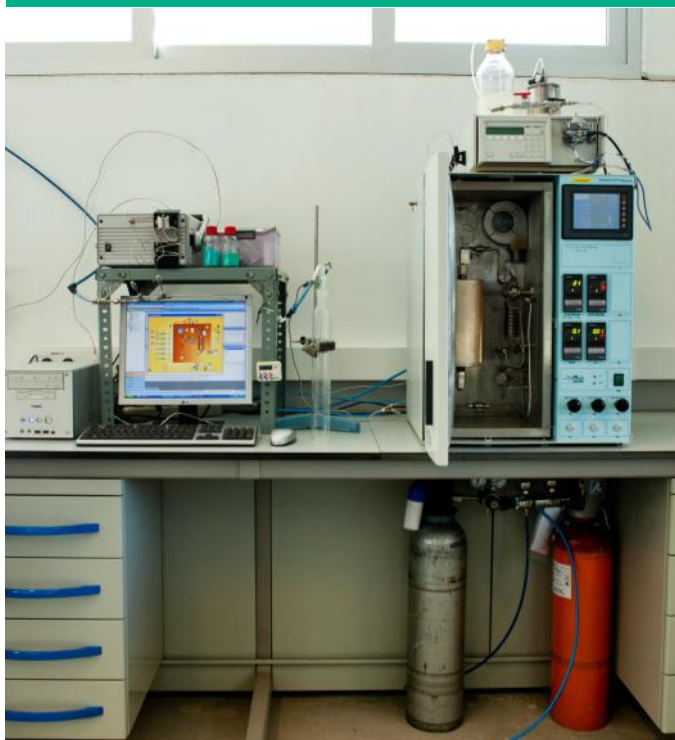
Figure 3: Micro-scale APR catalytic test rig at GPT-UNIZAR laboratories.
