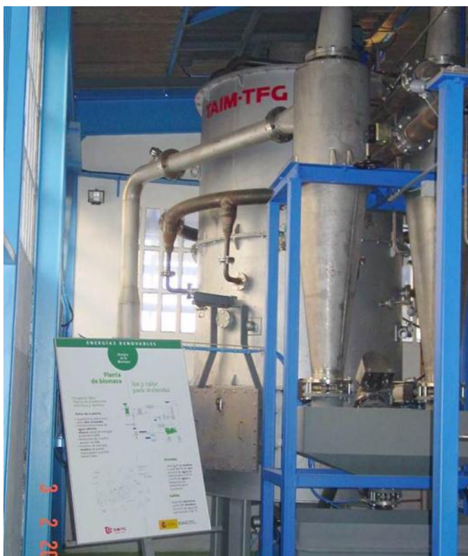
Figure 2: 700 kg/h biomass commercial-scale downdraft gasification plant at TAIM-WESER.
