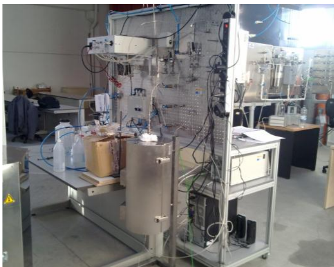
Figure 4: Lab-scale APR test rig at GPT-UNIZAR laboratories.
